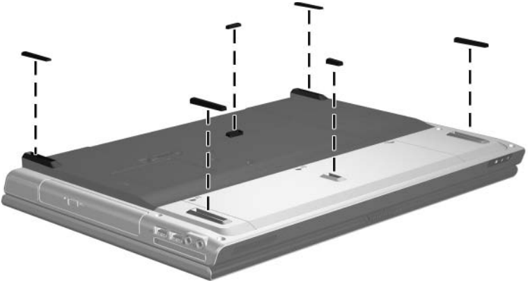
Replacing the Computer Feet
